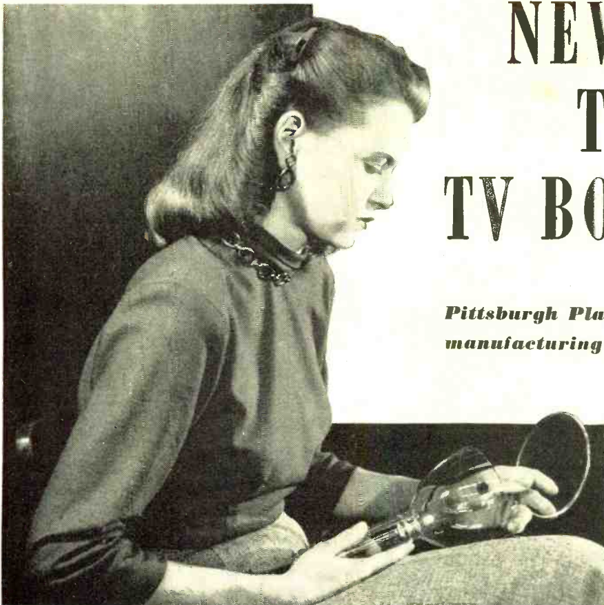
RCA's Caroline Tufts holds the newly developed Pittsburgh Plate Glass television picture tube face plate against the all-glass funnel to which plate is flame-sealed.
