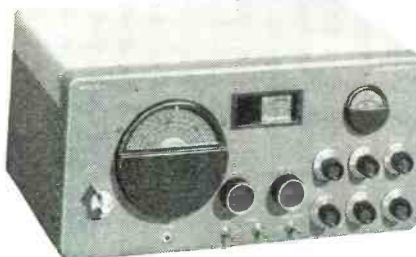
SX-43 All essential ham frequencies from 540 kc to 108 Mc. In the band of 44 to 55 Mc, wide band FM or narrow band AM, just right for narrow band FM reception is provided. $189.50
