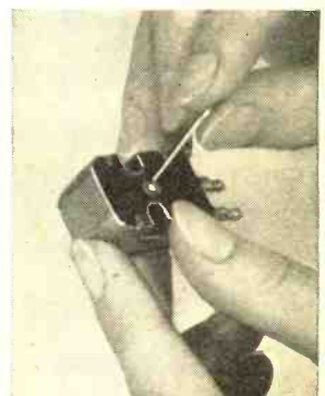
2 Use paper clip or wire to force stylus out of the cartridge.
