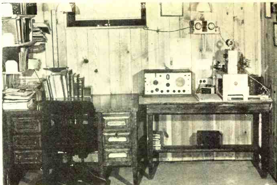
The four-foot table on the right holds a complete if modest ham station. A low-priced receiver is on the left end of the table, a home-made transmitter, built up breadboard style, on the right end. This cellar arrangement is neat and convenient and the radio equipment doesn't interfere with the study desk. A fine layout for the young student.
