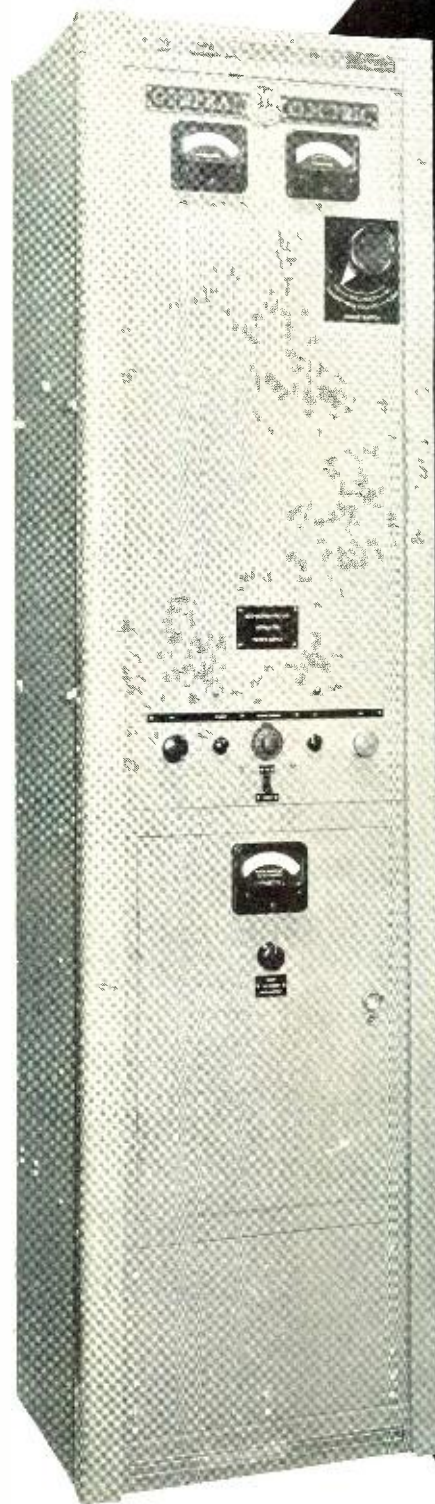
Fig. 1. Front view of the 500-50,000 volt regulated d.c. supply. A maximum output current of 1 ma. is available at any voltage within its range.
