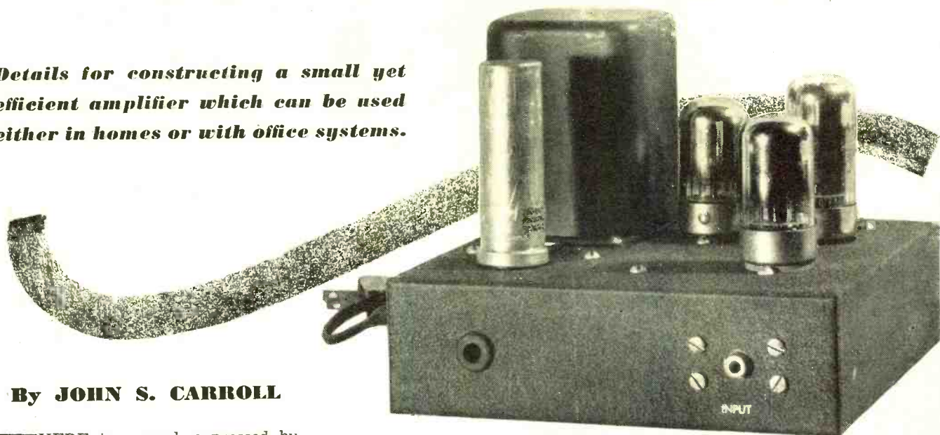
Fig. 1. External view of completed amplifier. The entire unit can be built on a 7" x 7" chassis. No tone controls were incorporated in this model, but may be added if desired.
